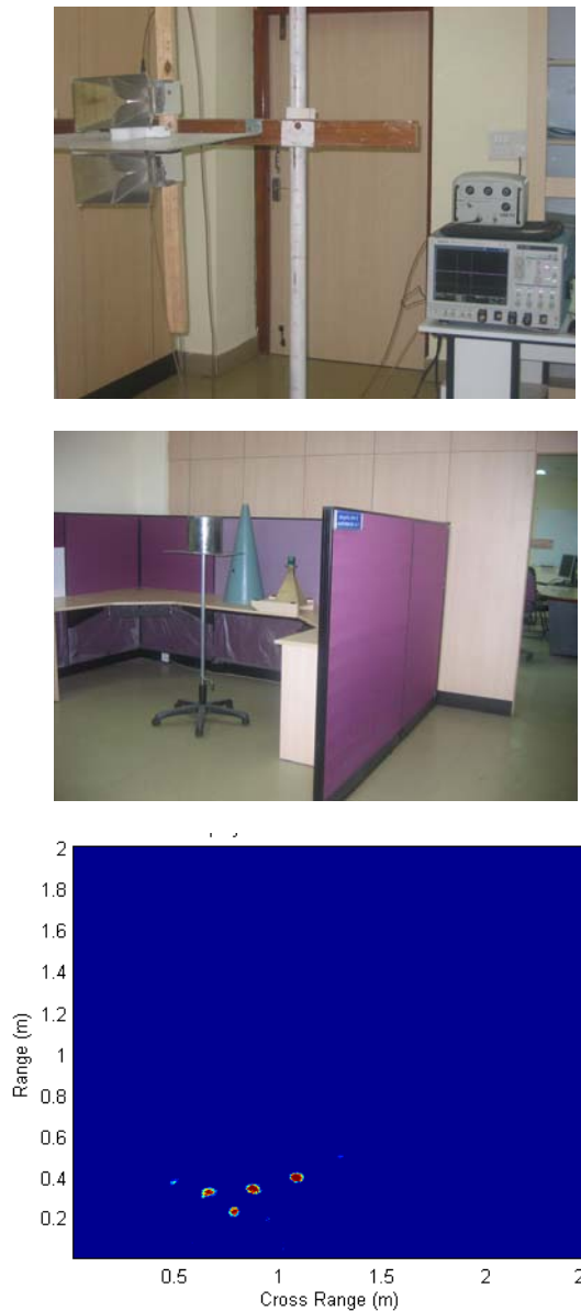
Figure 4. Experimental Data - Measurement Setup (top), Targets (middle) & Backprojected Image (bottom)
